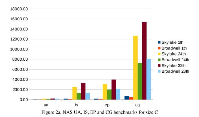
IS, EP, CG, SP and MG shows double the performance on the Skylake, which suggests that these codes are well vectorizable. The other benchmarks performance improvement is not as high, but, with increased core count it's still significant. The only exception is FT, where Broadwell performs slightly better. We will need to spend some time to understand this benchmark and explain this.
