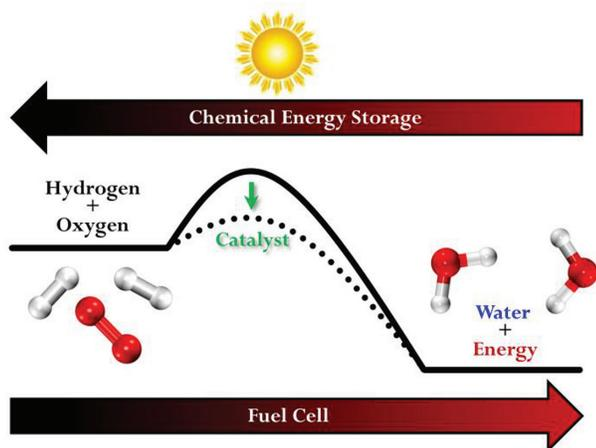
A traditional hydrogen fuel cell forms the basis of our approach. This cell combines hydrogen and oxygen to form water, along with a release of energy. This process is exquisitely environmentally friendly; the sole chemical by-product is water itself. Along the way, the chemical energy that is stored in hydrogen and oxygen bonds is released to power devices.
