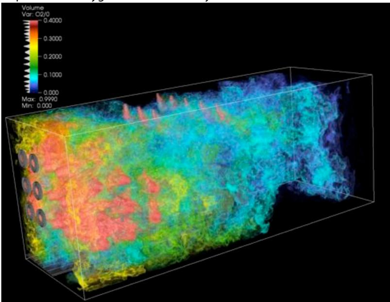
**Figure 3: Volume rendering of oxygen concentration inside the design boiler using LLNL's Visit software.**
