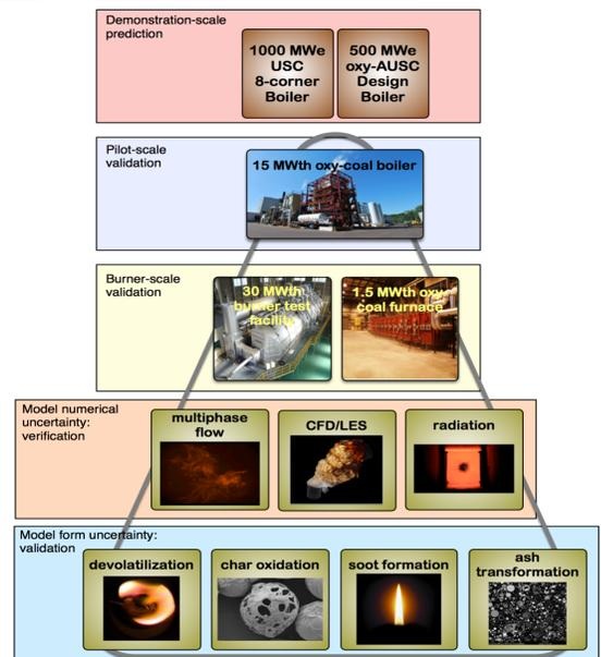
**Figure 1: Carbon-Capture Multidisciplinary Simulation Center validation hierarchy.**
